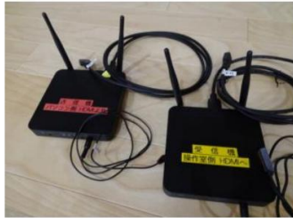
1 unit Used to send projection data from inside the hall to the control room Multipurpose hall
